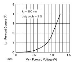
Figure 2. Typical High Current Forward Conduction Curve
