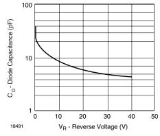
Figure 4. Typical Capacitance vs. Reverse Voltage
